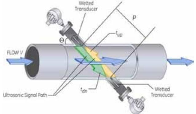
$$V = \frac{p^2}{2L} \frac{(t_{up} - t_{dn})}{t_{dn} \times t_{up}}$$
