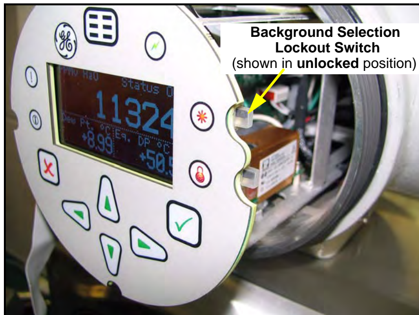
Figure 86: Background Selection Lockout Switch Location
