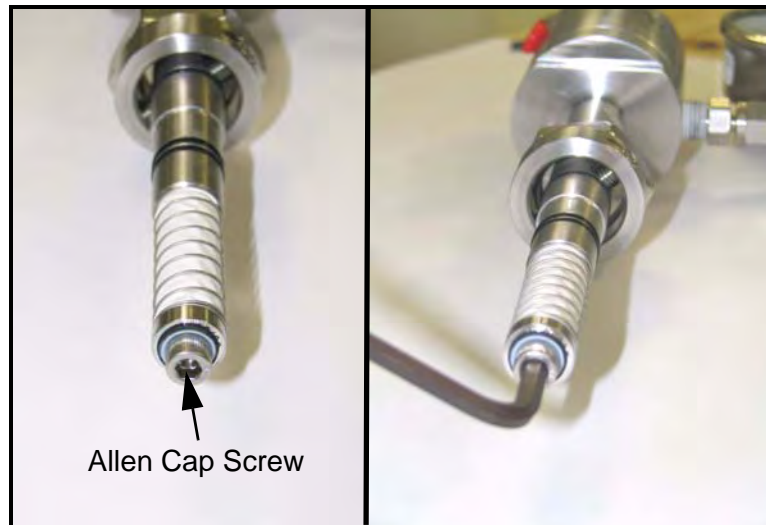
Figure 15: Checking/Tightening the Allen Cap Screw
