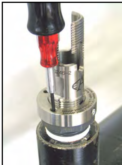
Figure 14: Tightening the Allen Screws
