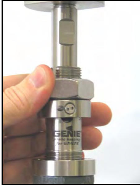
Figure 21: Tightening the Insertion Nut
