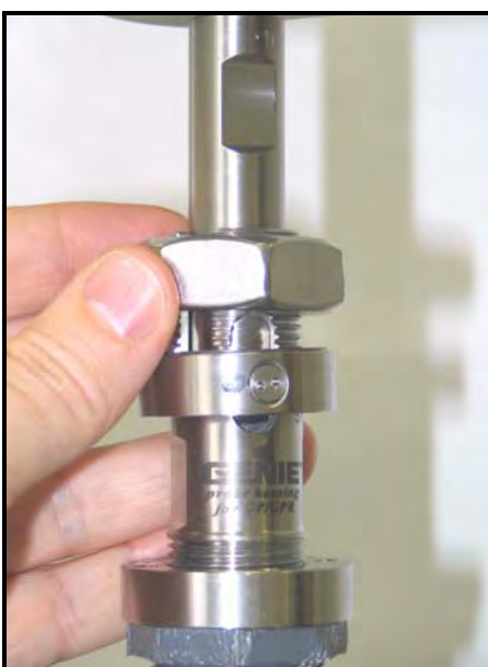
Figure 20: Loosening the Insertion Nut
