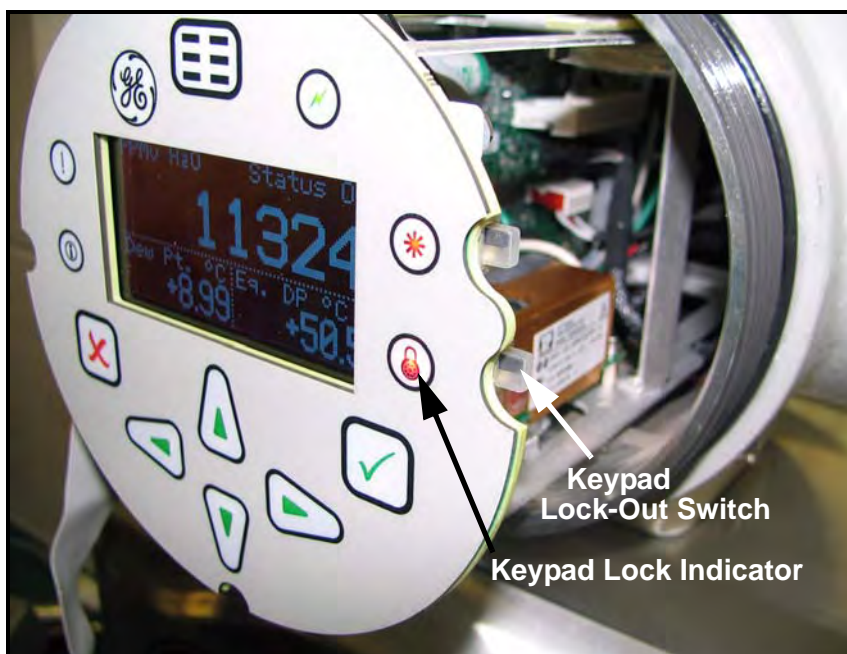
Figure 36: Keypad Lock-Out Switch Location
