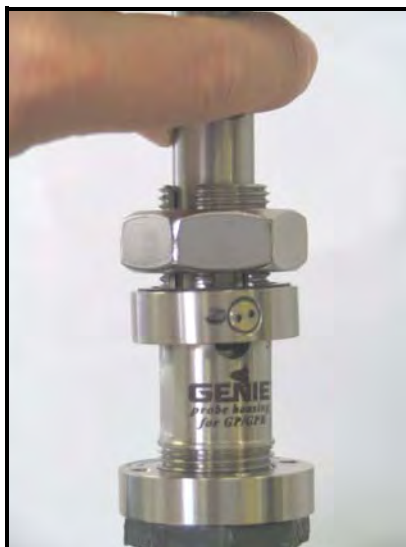
Figure 19: Rotating the Probe
