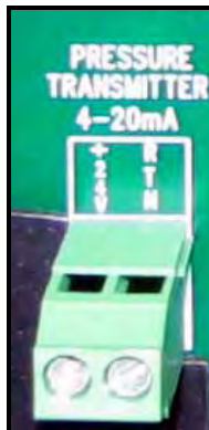
Figure 28: Pressure Transmitter Connections
