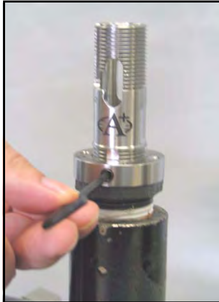
Figure 13: Aligning and Tightening the Allen Screw
