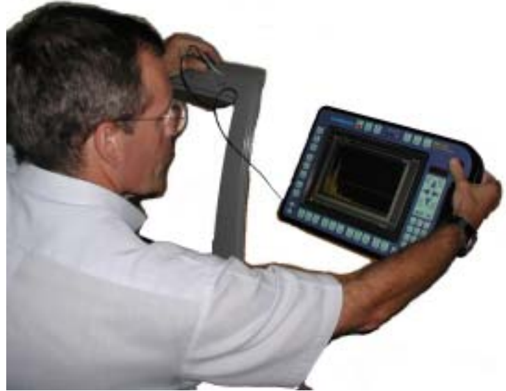
Glue bond evaluation in the automotive industry
