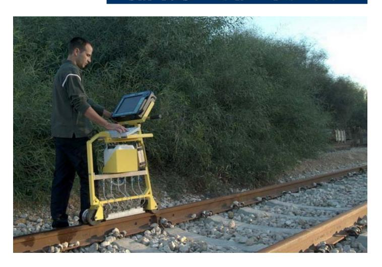
State-of-the-art ultrasonic inspection system for manual flaw detection, evaluation and documentation of defects in train rails
