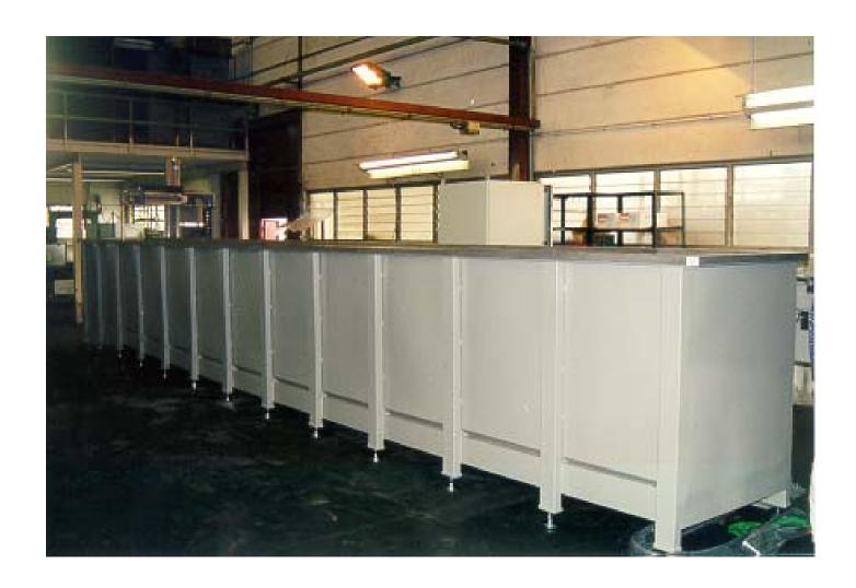
Precision inspection systems for C-scan imaging, evaluation and documentation of flaw indications in extruded billets or bars
