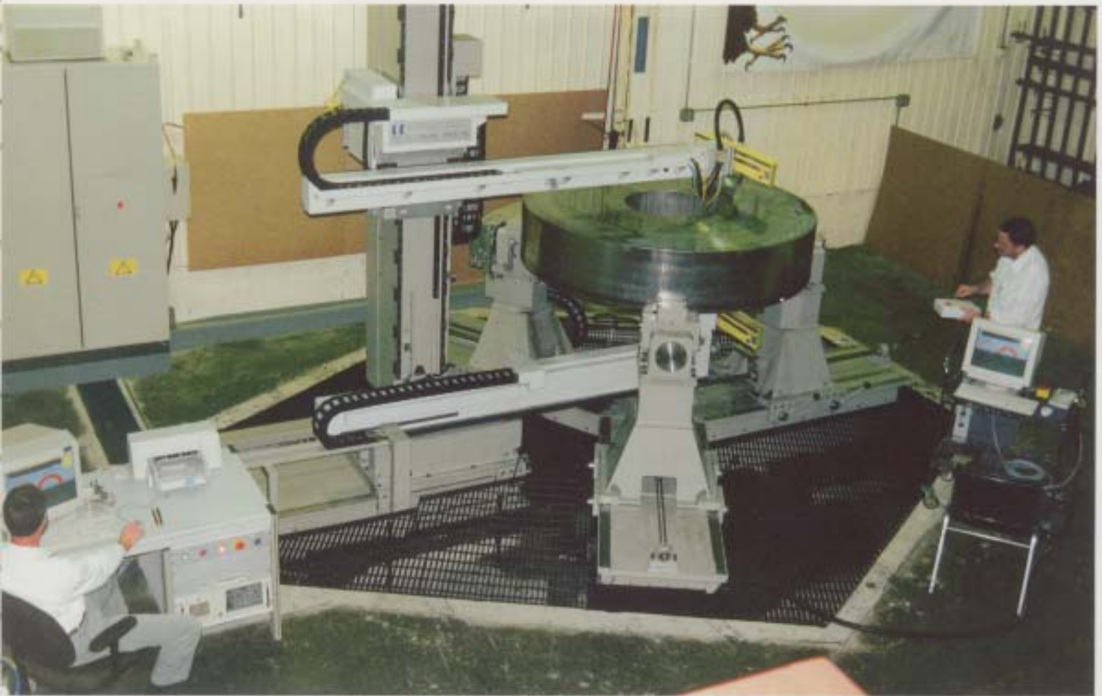
Dual-beam search tubes for simultaneous P-E and T-T inspection
