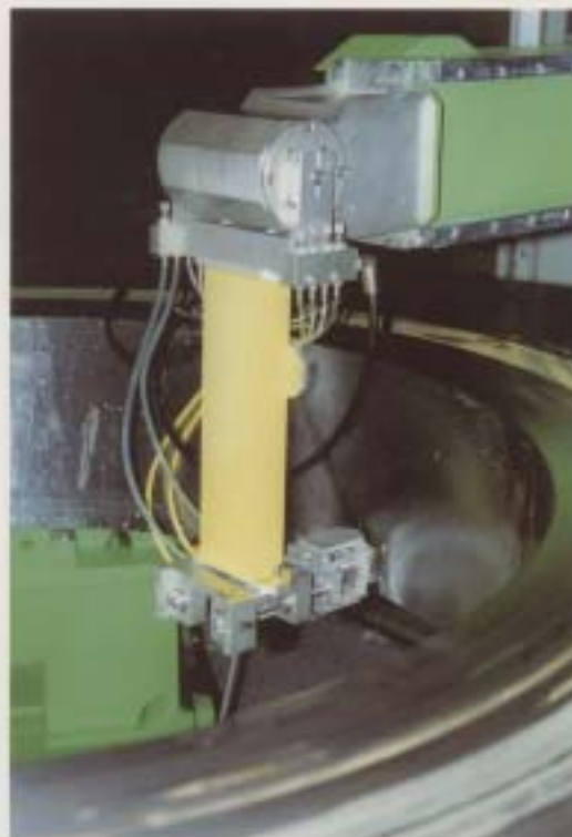
Extension arms for bore inspection
