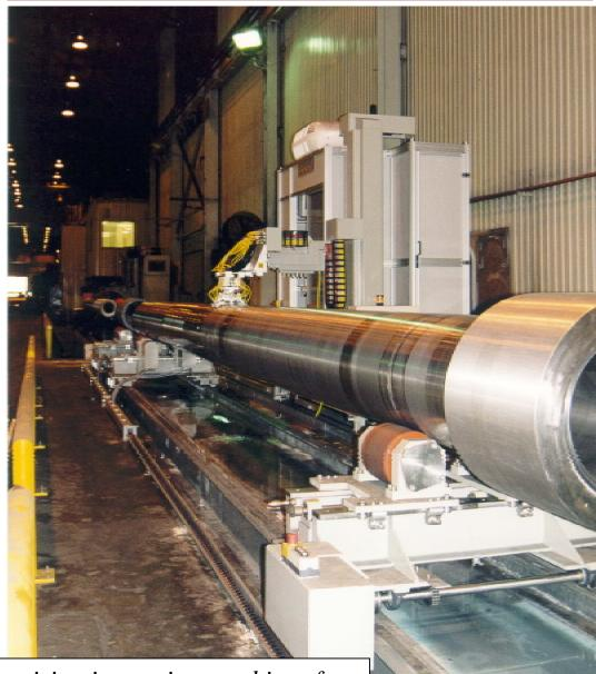
High-speed, precision inspection machines for detection, evaluation and documentation of flaws in large, thick-walled tubulars
